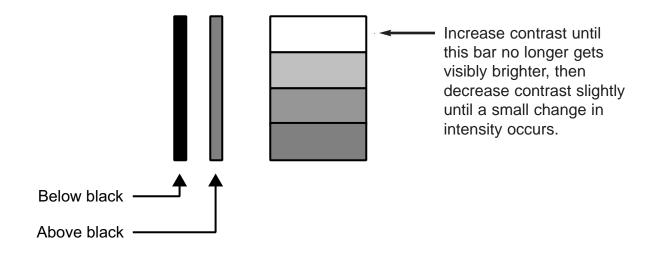
**<u>CONTRAST</u>** adjusts the white level of the image.Adjust contrast until there is a distinct definition between the two brightest bars.
